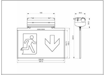
Control System: SmartZ Luminaire: Self-Contained
